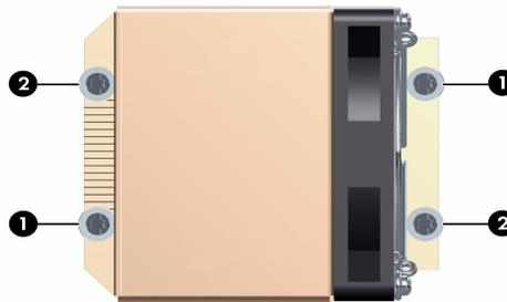
Figure 5 Tighten heatsink screws
